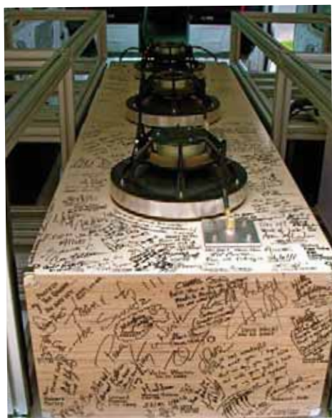
The subwoofer enclosure is built from 2.83"-thick Baltic Birch ply. Note the many autographs of world-famous musicians who have heard the Magic Bus.
