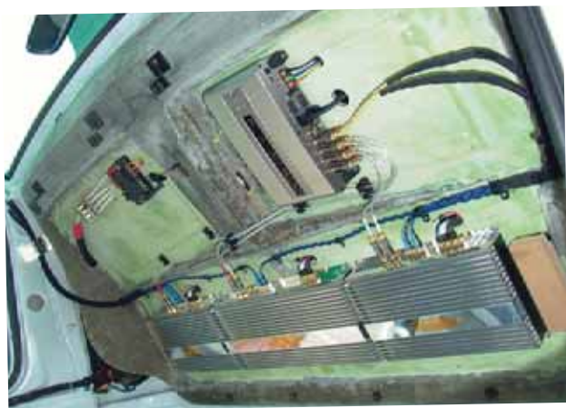
View of overhead electronics console (cosmetically unfinished) with headliner removed.
