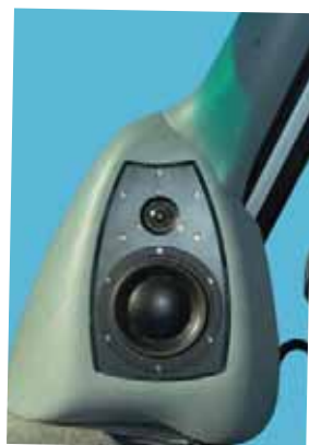
left: The front monitors are housed in custom enclosures. above: The door panels were built from scratch to house the lower-midrange driver (cosmetically unfinished).
