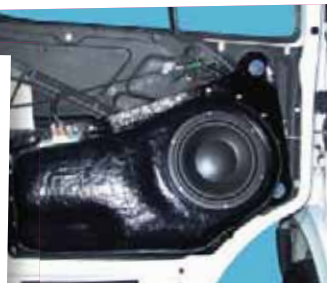
left: The front monitors are housed in custom enclosures. above: The door panels were built from scratch to house the lower-midrange driver (cosmetically unfinished).
